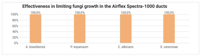
Test of fungistatic properties of the polymeric material in a 28-day test. The presented values may include a deviation resulting from the applied measurement method (0.1%).
