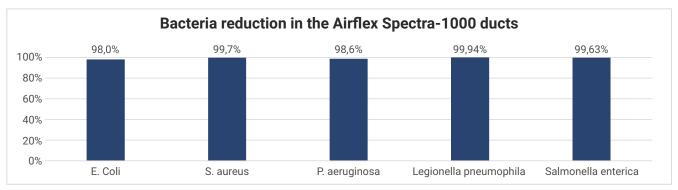
Test of antibacterial properties of the polymer material in a 24 h test. The graph shows the bacteria reduction degree after 24 h contact with the Airflex Spectra sample.
