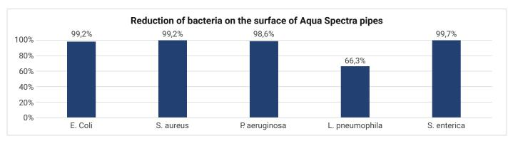
Test of antibacterial properties of the polymer material in a 24h test. The graph shows the degree of bacterial reduction after 24h of contact with the Aqua Spectra sample.
